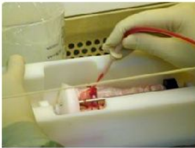
Seeding the cells in the InBreath bioreactor
